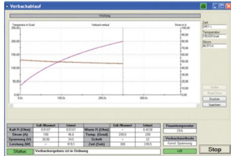
**Bonding with constant voltage – constant-voltage method**
