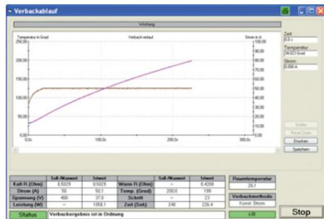
**Bonding with constant current – constant-current method**
